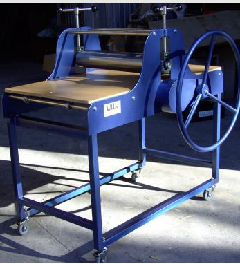
This press is for serious print makers, they are all Reduction Drive with a gear Ratio of 3:1. This gear reduction model has a roller chain from the hand wheel via the reduction to the bottom roller, this requires less effort to drive the bed through the rollers. The press comes complete with heavy duty shafts, bearings, and a stand with Castors as standard.
